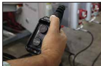
Hand-held pendant controls all height and pulling operations
