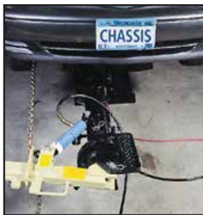
Exclusive Tilt 'N Turn tower allows pulling from multiple angles, 360° around vehicle
